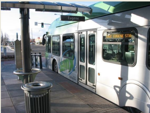
The EmX in Eugene is an example of a full BRT system, which is distinguished by its use of exclusive street right-of-way or grade-separated running ways.
