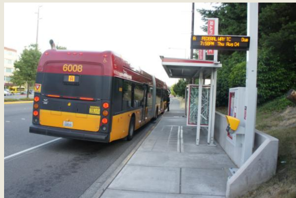
The RapidRide service in the Seattle area is an example of Rapid Bus service. It runs in mixed traffic with transit priority features, but has branded, stylized vehicles and some well-developed station features.
