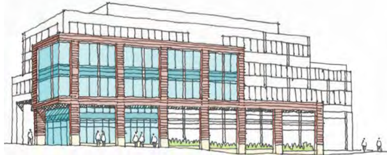
Figure 24: Masonry or pre-cast outer skin wraps around the bulk of an office building adding a richness of texture, durability and detail where the building meets the street.
