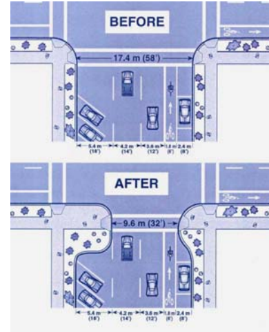
Curb Extensions - Before and After
