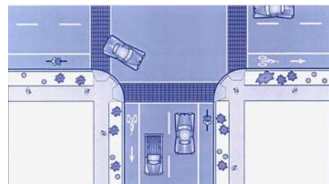
Patterned Crosswalk at Intersection
