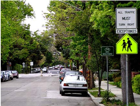
Figure 5.4 A non-motorized only crossing forces motor vehicles to turn at an intersection
