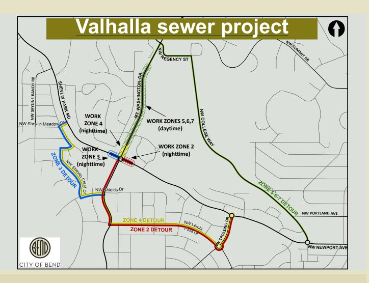
To control sewer odors in the Valhalla neighborhood, the City of Bend is about to build a new sewer line in the Valhalla neighborhood area. Crews will install new sewer piping down Mount Washington and along Shevlin Park Road, and will build an odor control facility near the roundabout. Upon successful completion of the project, the City will be able to stop using expensive chemicals to control odors.
