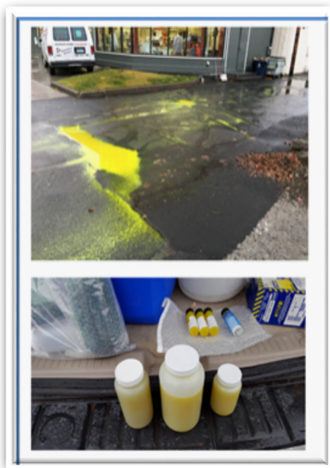
One of multiple downtown spill locations and lab samples taken one morning as part of investigation of spill that was tracked upstream. Conclusions indicate probability of improper disposal of paint in the garbage and leakage during transport.
