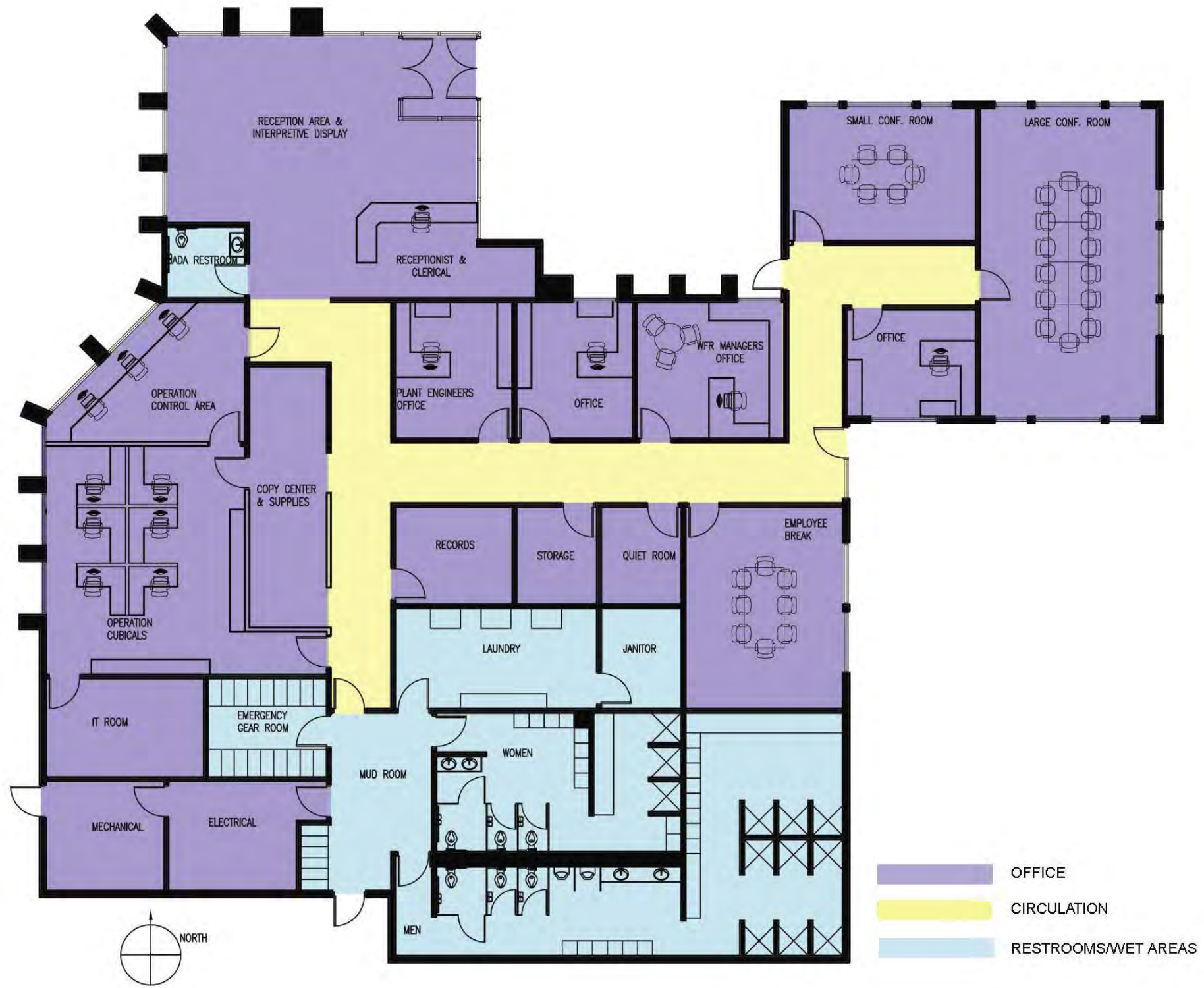
Figure 6 Proposed Operations Building Renovation
