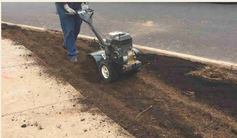
Deep incorporation of amendment to improve poor soil conditions. Be sure to sweep excess dirt and debris from streets and sidewalks.
