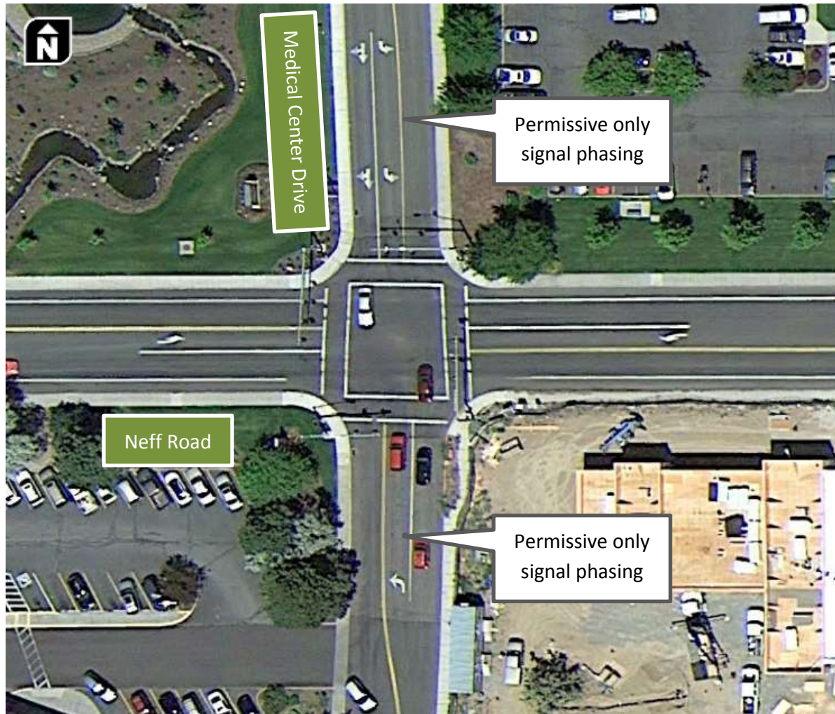
Figure 13. Neff Road/Medical Center Drive intersection configuration.
