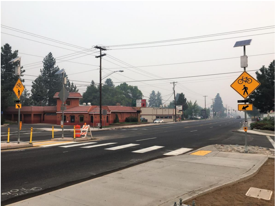
Figure 1. Example of a Rectangular Rapid Flashing Beacon (RRFB)
