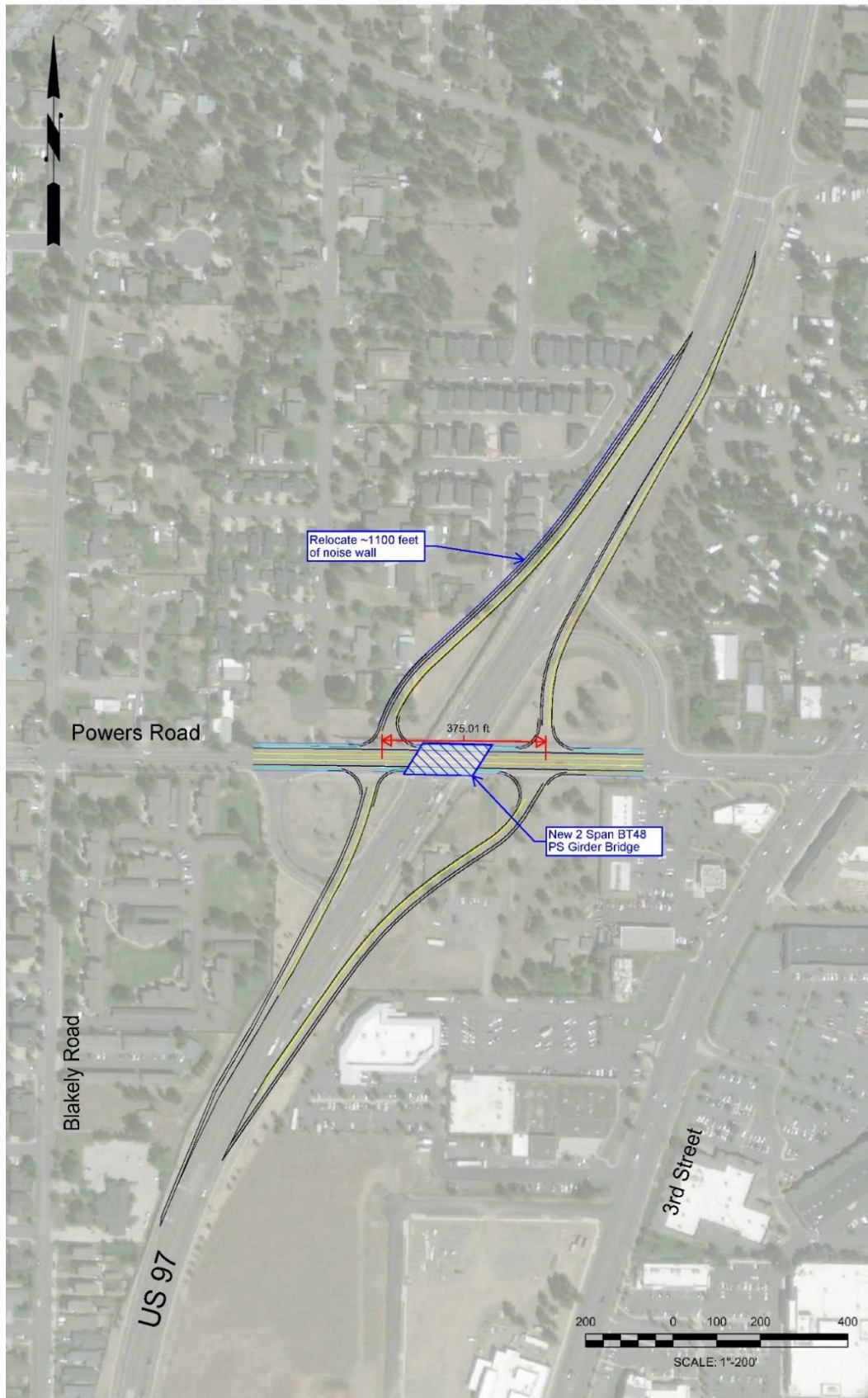
Figure 1: US 97/Powers Road Tight Diamond Interchange Concept
