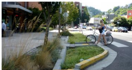
Mid-block crossing, curb extensions, stormwater treatment
