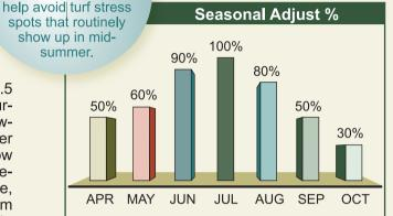
Most irrigation controllers have a Seasonal Adjust % feature that allows the user to easily increase / decrease runtime minutes for all zones. Adjusting the percentage will add or remove runtime minutes to ALL irrigation zones. Use the bar chart as a guide to make changes to your irrigation schedule each month.
