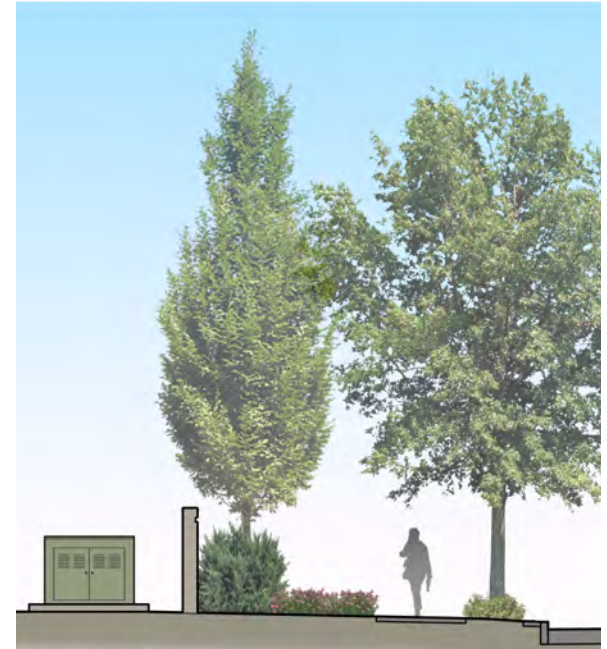
Figure 15: Walls or screens should be tall enough to obscure utilities, loading areas and work areas. Shrubs should be massed in front of the wall for further screening and to soften the wall's appearance.
