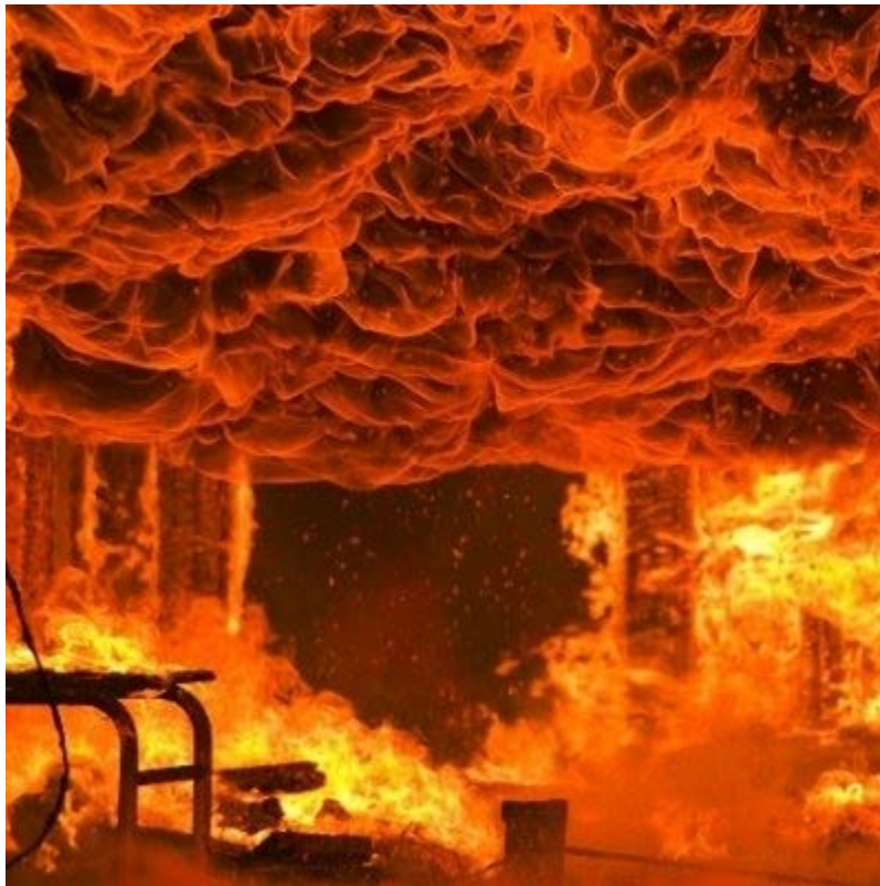
Flashover, courtesy of Life Safety Services
