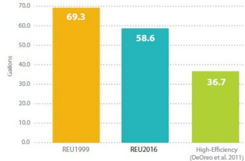
Figure 7. Indoor average gallons per capita per day, REU1999, REU2016, High Efficiency Studies
