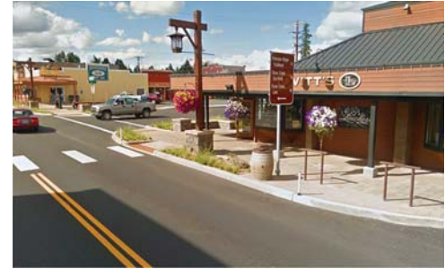
Example of traffic calming treatments on an arterial street. Notice curb extension, light post, trash barrel, hanging flower baskets, and other vertical elements near street. Image ©2016 Google.
