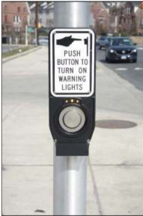
Figure 3. Example of pedestrian pushbutton and R10-25 sign with pilot light for pedestrian actuation.
