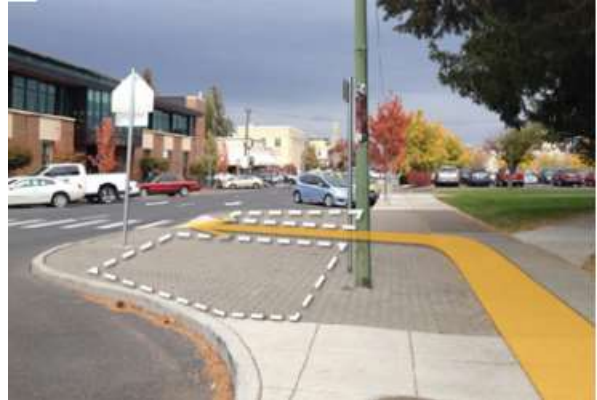
Figure 61 - Curb Extension Area for Bike Parking
