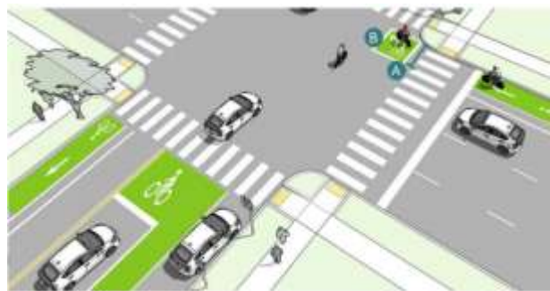
Figure 42 A bike box on the near side and a two-stage left turn box on the far side of the intersection.
