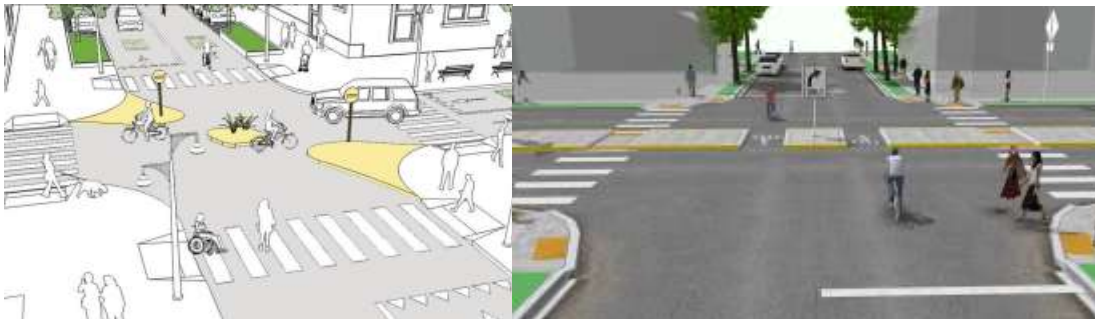
Figure 56 - Modal Filters (Diagonal Example from National Association of City Transportation Officials (NACTO) Global Street Design Guide, 2016 and median example from NACTO Urban Bikeway Design Guide, 2014)
