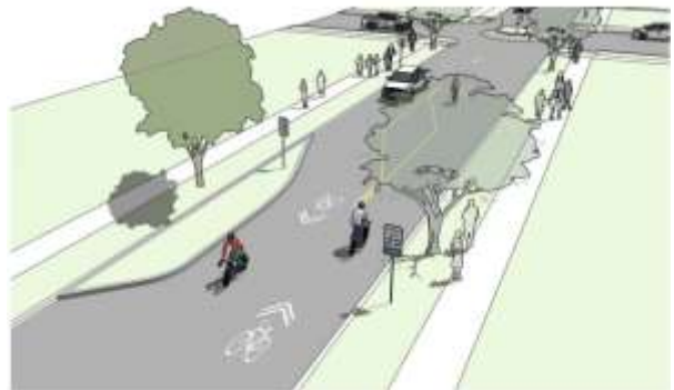
Figure 29 - Image from NACTO Urban Street Guide that shows a neighborhood greenway with traffic calming.
