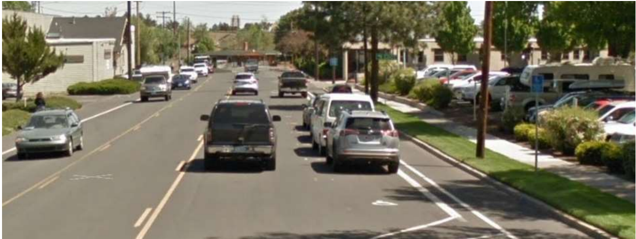
Figure 20 - Parking Separated Bike Lane
