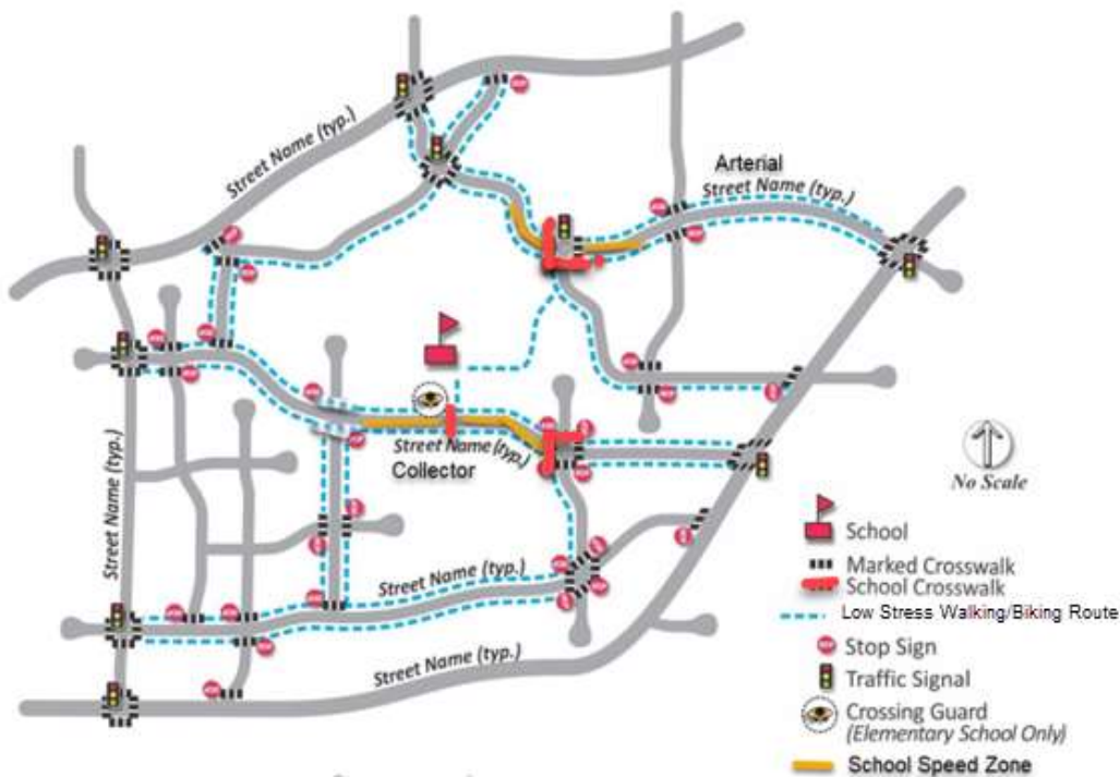
Figure 34 - Example Safe Routes to School Plan. Modified from Clark County School. Zone Traffic Control Policy, Clark County, December 2016
