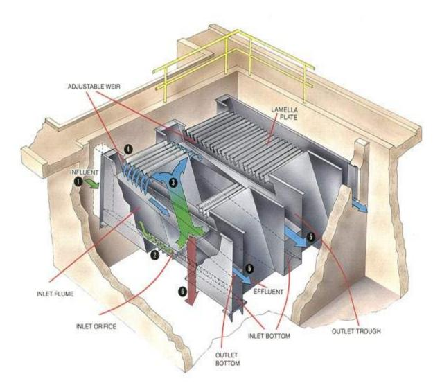
The material costs for the plates or tubes can vary depending on the materials required for the installation. Solids loading on surfaces and removal of solids can be a problem in some configurations. Similar to conventional sedimentation, 30 minutes or more of detention time in the flocculation process is necessary. Plate and tube settlers have been in use for many years in water treatment and are a widely accepted technology for settling of flocculated solids.
