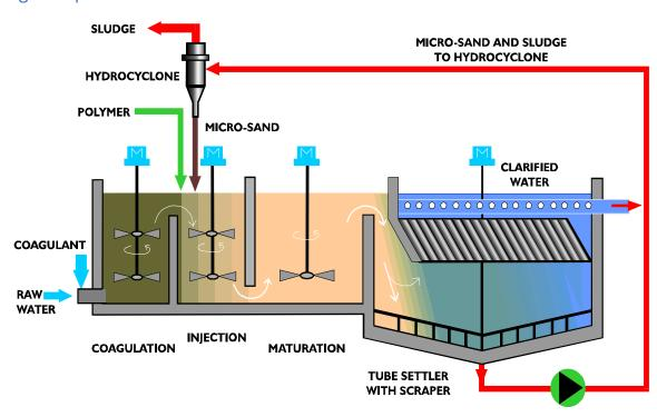
Figure 6 | Schematic of the Ballasted Sedimentation Process
