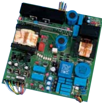
Electronic ballasts ensure that the Spektrotherm® HP UV lamps operate cost-effectively
