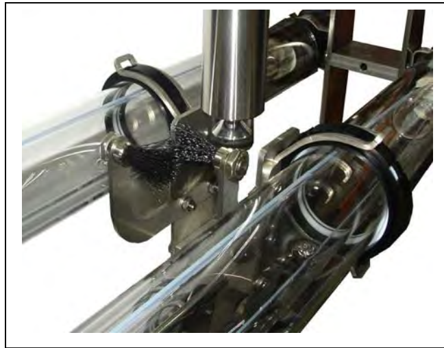
Fig. 2 Wiper rings and sensor cleaning brushes
