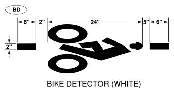
Install in Type B - HS Preformed Thermoplastic Place marking in optimal location for bicycle to actuate the traffic signal.
