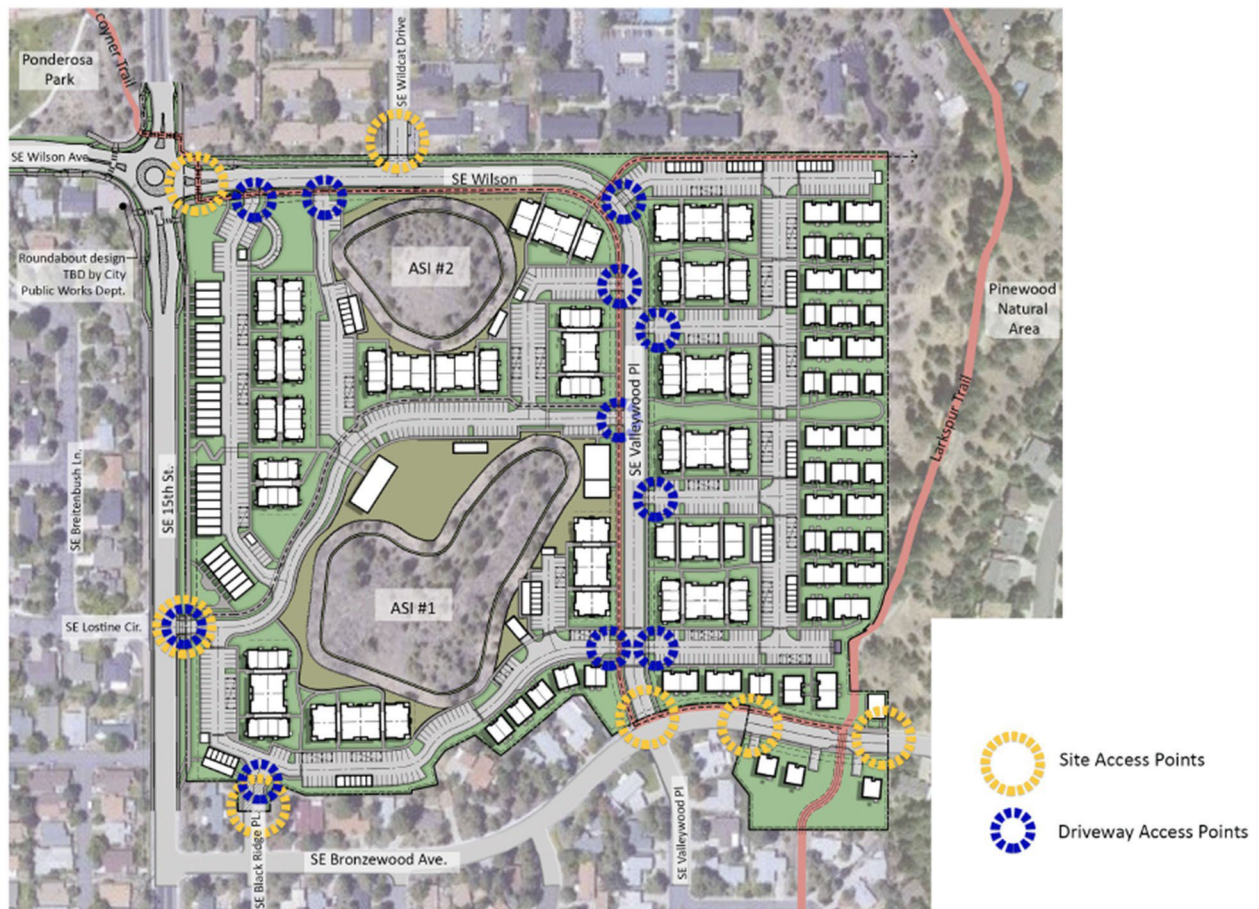
Figure 2.7.3150.B. - Vehicular Access Diagram
