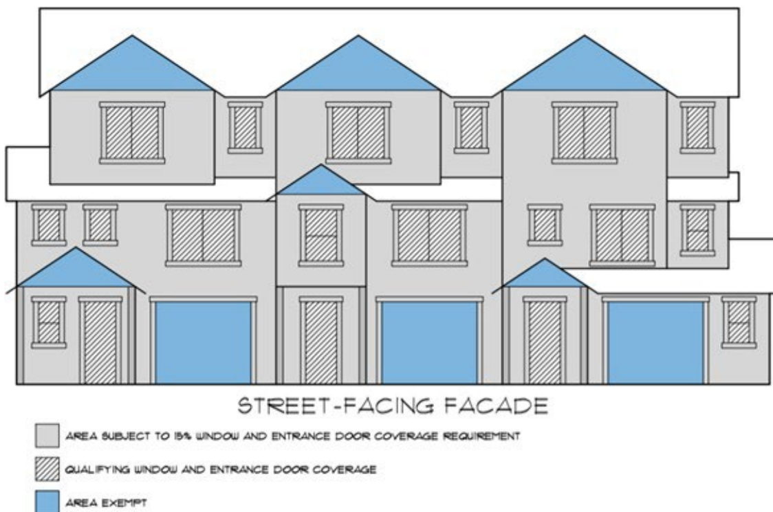
Exhibit 2.7.3145 – Calculation of base wall area for 2.7.3145.E.2.b.
