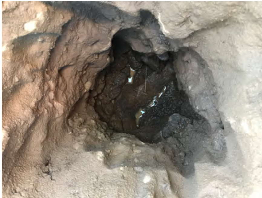
Figure 5. Hole #2 with what appears to be weathered basalt bedrock in bottom.
