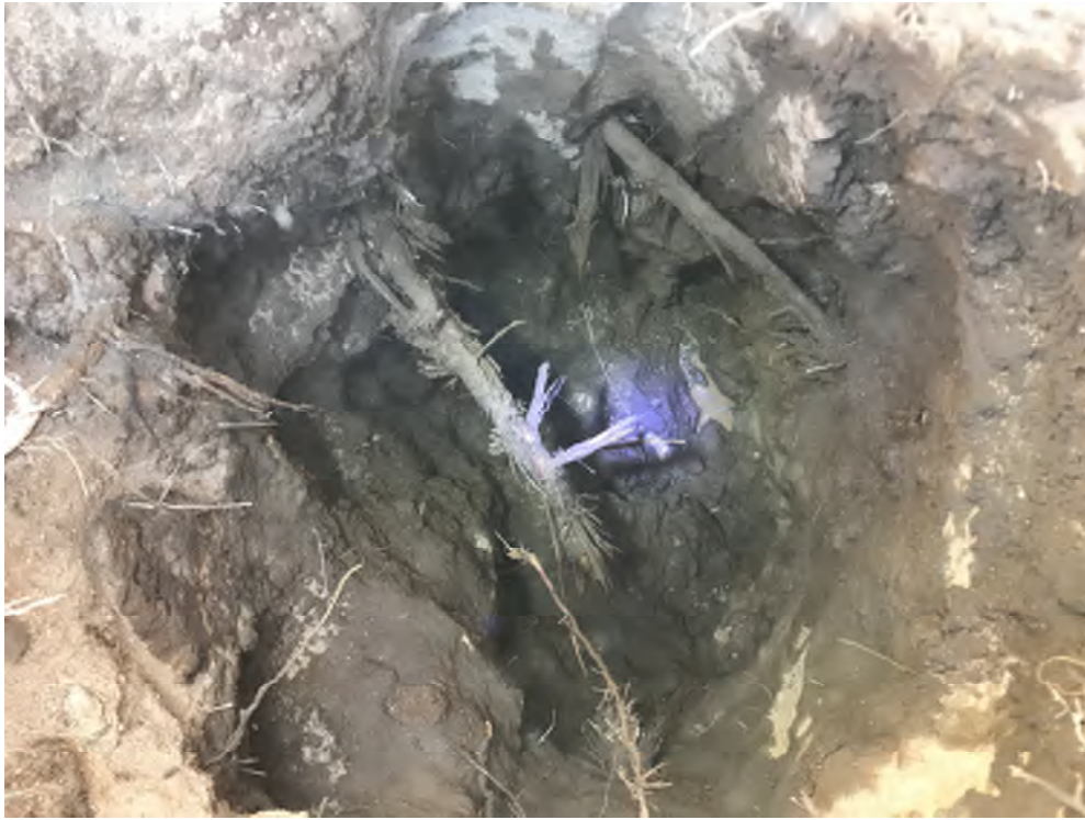
Figure 6. Hole #3, with what appears to be weathered basalt bedrock in bottom.
