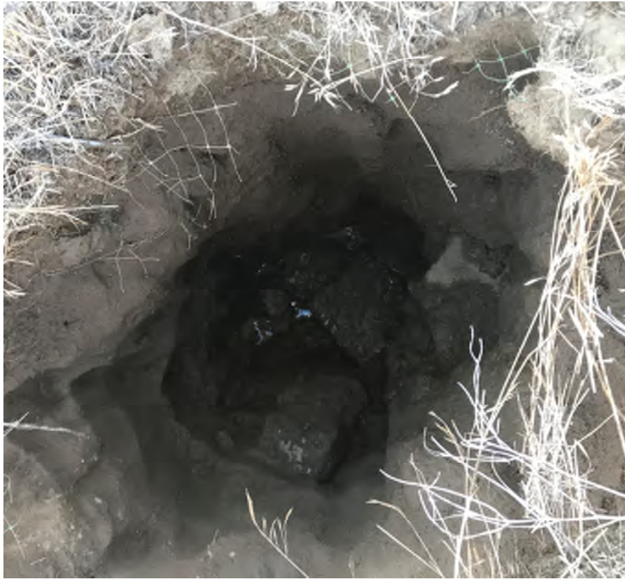
Figure 4. Hole #1 with what appears to be rubble fill.
