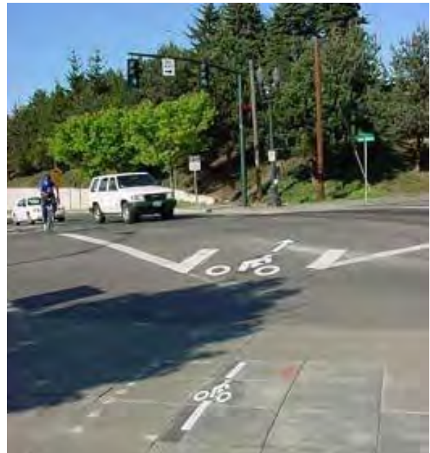
A bicycle detection system triggers a change in the traffic signal when a bicycle is detected.
