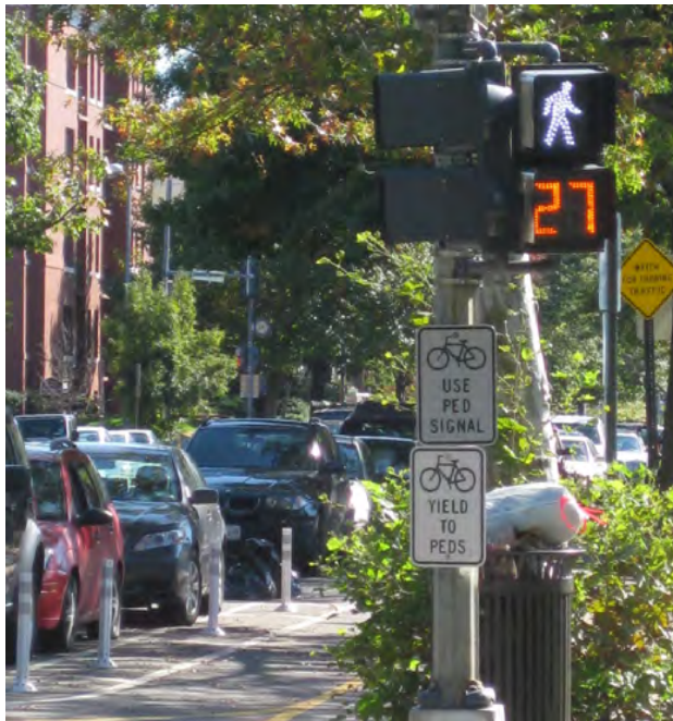
A bicycle signal head at a signalized crossing creates a protected phase for cyclists to safely navigate an intersection.
