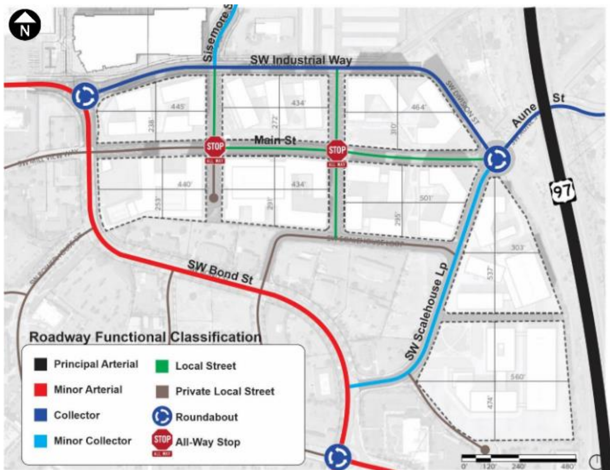
Figure 12. Recommended Vehicular System Classification and Traffic Control (Source: Timber Yards Master Plan)
