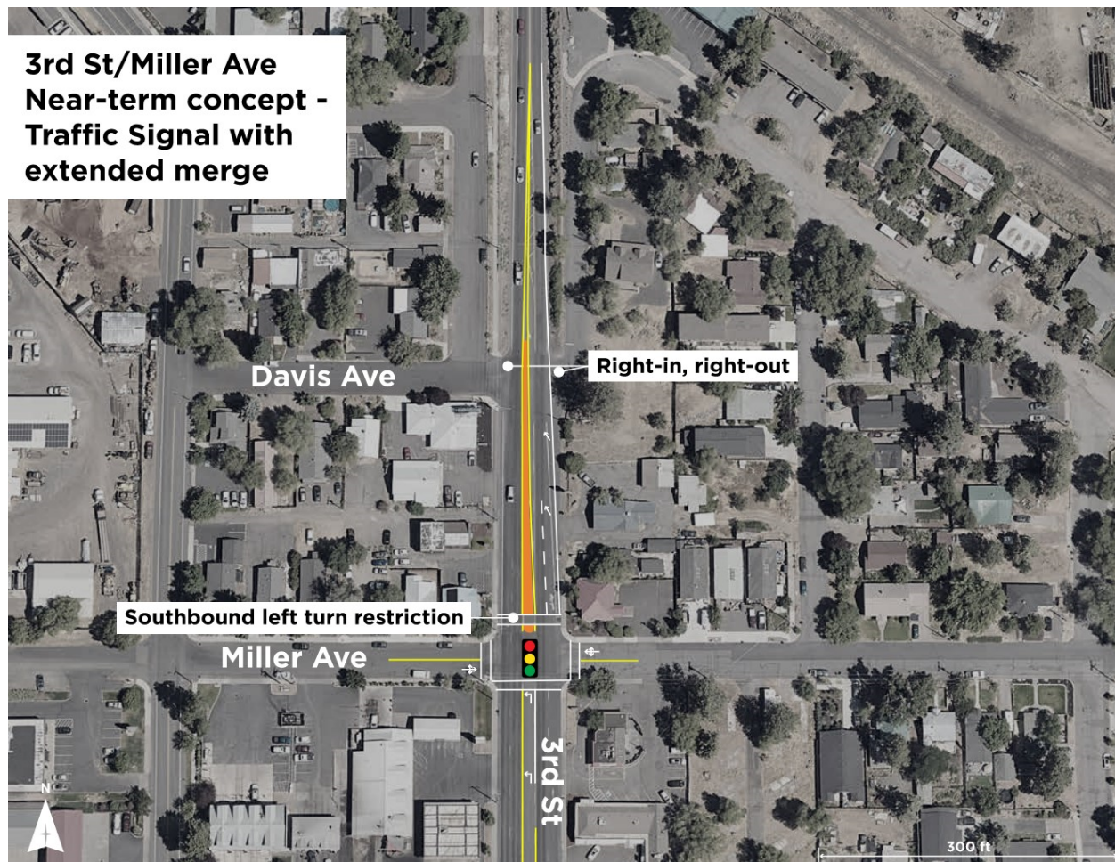
Figure 4. Alternative B.1 Traffic Signal at 3rd Street/ Miller Avenue
