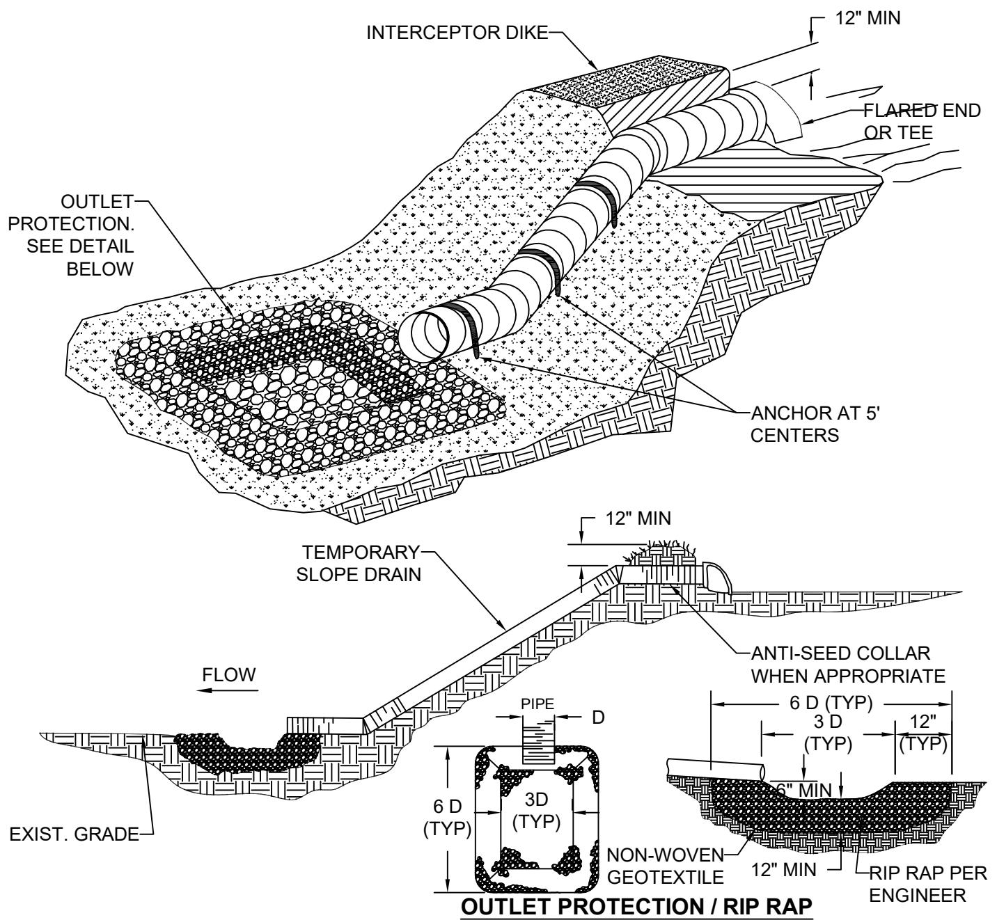
GRADE RIPRAP SHALL BE THE CLASS AND SIZE OF ROCK ACCORDING TO THE FOLLOWING:
