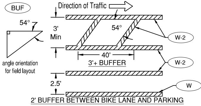
Install buffer stripes in thermoplastic / horizontal stripes parallel with traffic in paint
