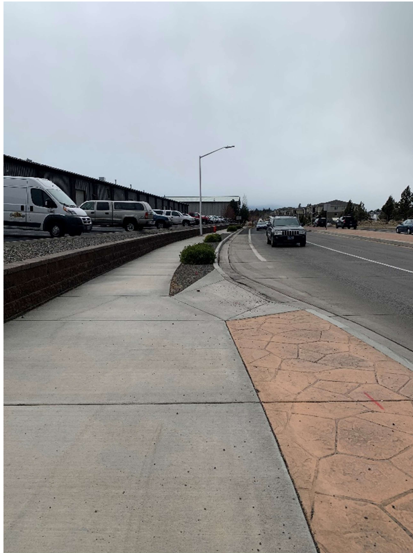
Figure A-1. The bike lane ends appropriately at the ramp. In this photo, the curvature helps reinforce the bike rider's choices of merging into the traffic lane or exiting onto the shared-use path and is a good example. The shared-use path, however, should have been extended further, to get past the bike ramp, so someone walking with low vision doesn't easily walk down the bike ramp.
