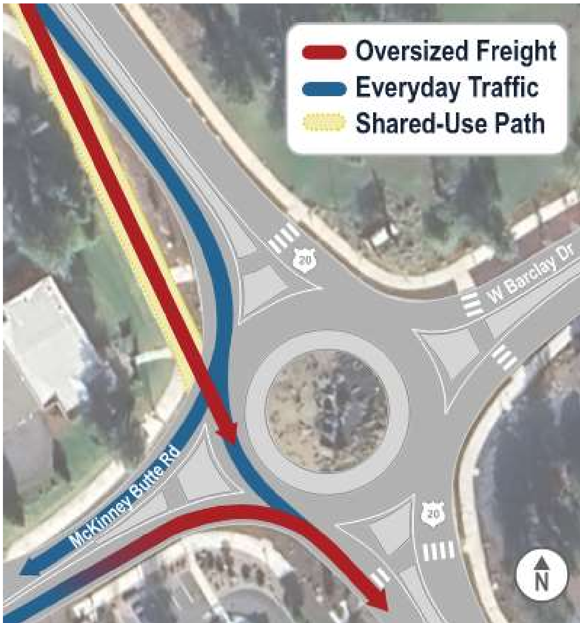
Figure 14. The roundabout on US 20/Barclay Drive in Sisters, Oregon, uses a separate path of travel for oversize freight. The shared-use path has been widened and strengthened to allow oversize/overweight freight to approach the roundabout on a tangent approach, while everyday users approach on a curvilinear path to manage entry speeds.
