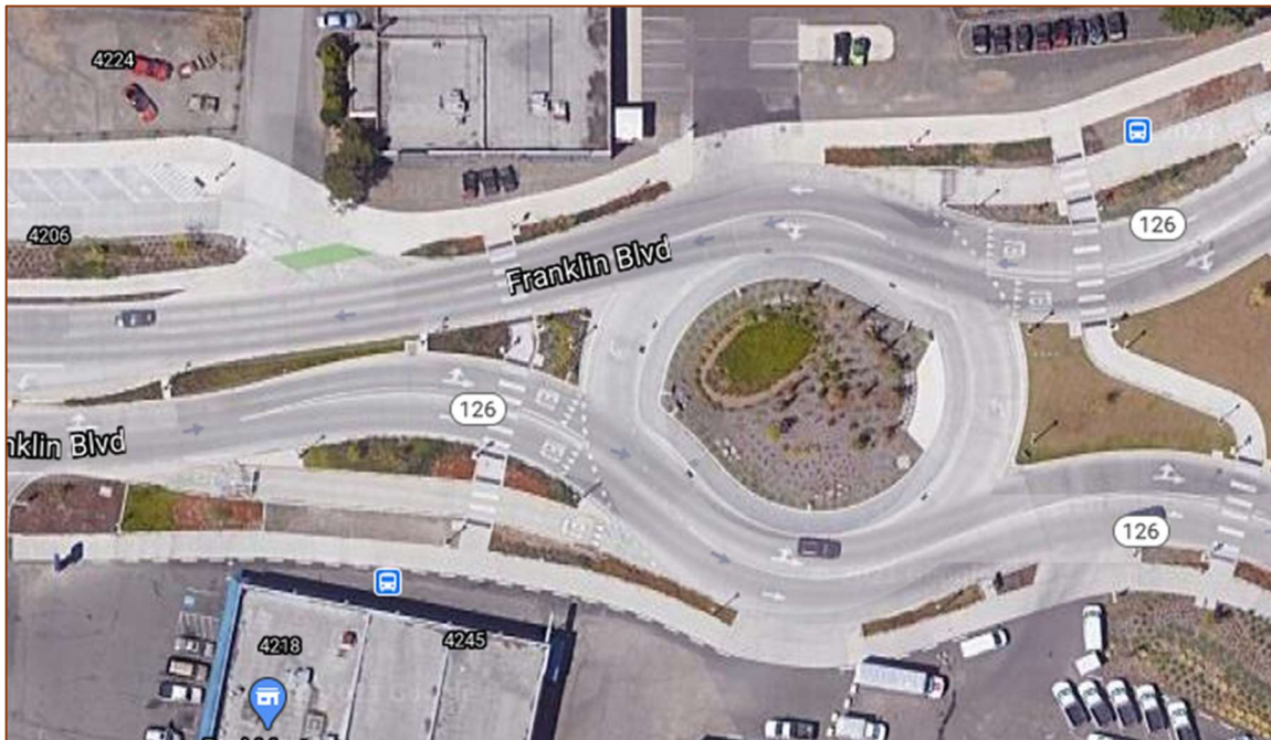
Figure 24. An example of a nested lane addition in Springfield, Oregon on US26 and Franklin Boulevard. This can improve lane discipline without the use of a spiral and reduce the size of the roundabout.
