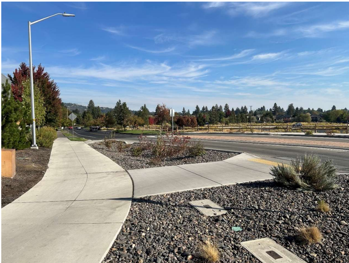
Figure 17. Longer crosswalk approach to the detectable warnings facilitates longer bikes waiting out of the shared use path and allows people driving to see that people are turning to cross the street. Northbound Columbia at Simpson. This design provides ~15feet between the domes and path.
