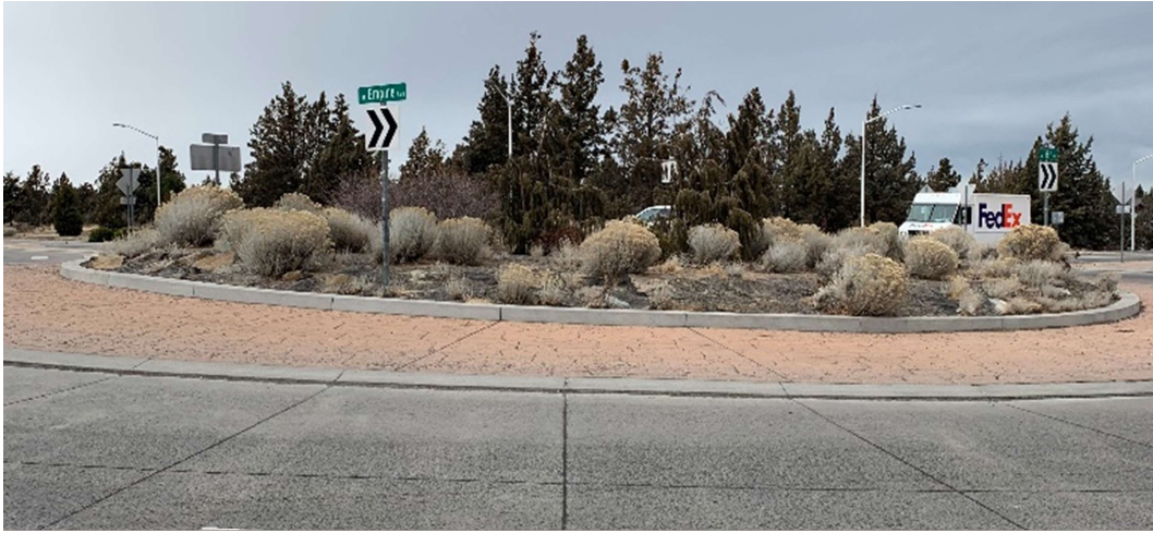
Figure 34. An elevated and landscaped central island slows vehicles and queues drivers to turn by creating a terminal vista.
