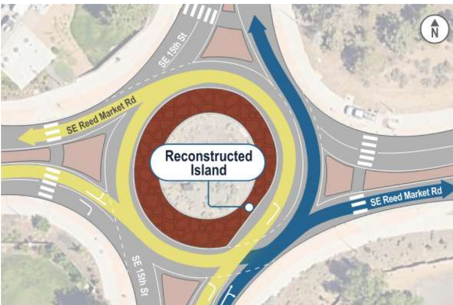
Figure A-8. To fix this issue, the central island truck apron needs to be partially reconstructed as shown in this exhibit to create the needed spiral. The central island curbing would do most of the work to enforce the spiral movement, and this would be reinforced with spiral striping on the pavement.
