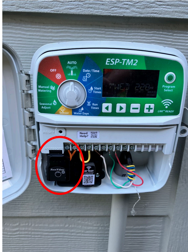
Smart Link installed in new controller
