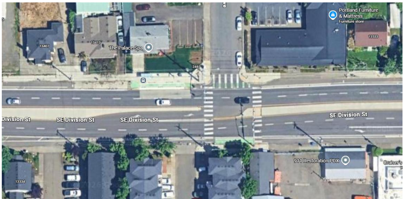
FIGURE 22: EXAMPLE OF A RIRO MEDIAN WITH PEDESTRIAN CUTS AND A MAJOR STREET LEFT-TURN ALLOWED
